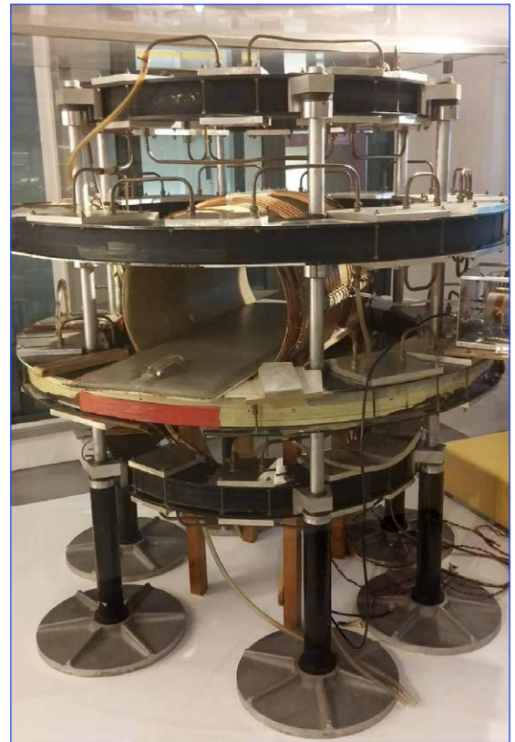
The first MRI scanner built and used, in Aberdeen Royal Infirmary in Scotland.
