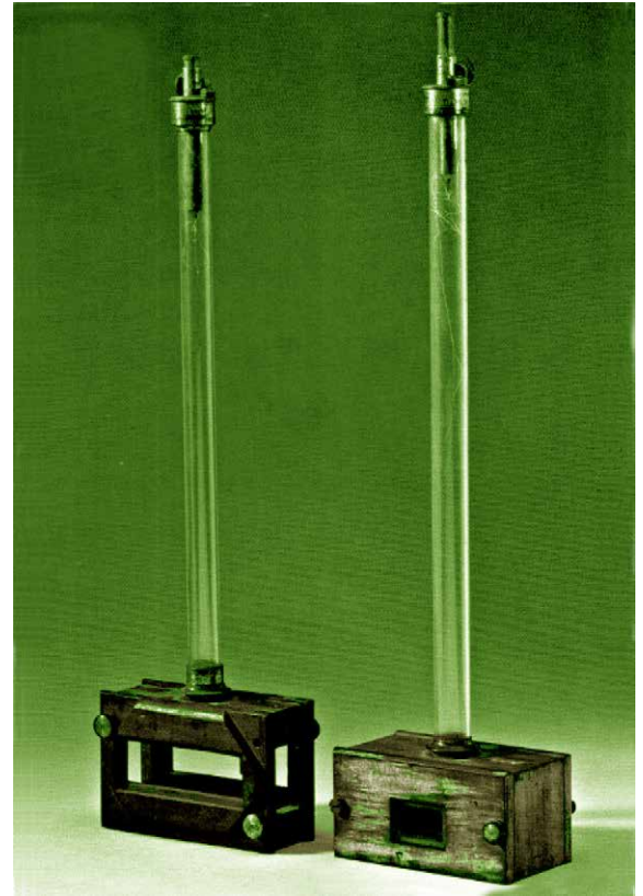
A pair of mounts for air thermometers used in an absolute zero experiment
