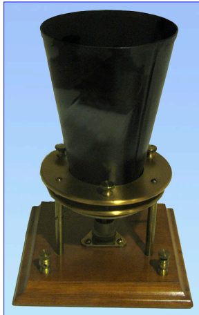
The liquid telephone that transmitted the first complete sentence over a wire on 10th March, 1876
